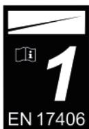
Refers to bicycles and EPACs used on normal paved surfaces on which the tires are intended to maintain ground contact at average speed, with occasional drops.
