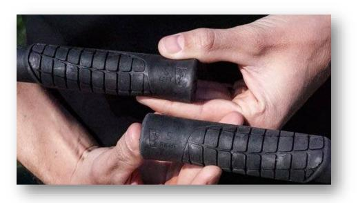
Assume the riding position by placing your hand around the handlebars and memorizing/marking the position of the Edge of the hand.
