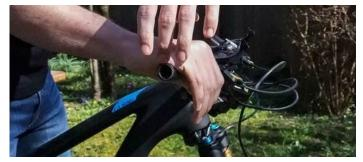
Place the middle row of knobs of the 711 R on the outside at the level of the marking and note the orientation of the grip to the handlebars.
