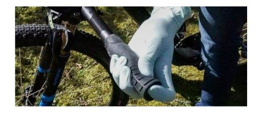
Last, small alignments are still possible for a short time. **Tip:** At the height of the middle row of knobs, you can see across, very faintly, the shape dividing line of the grip. If this is straight and the middle row of knobs is in the right place, the grip is optimally positioned!
