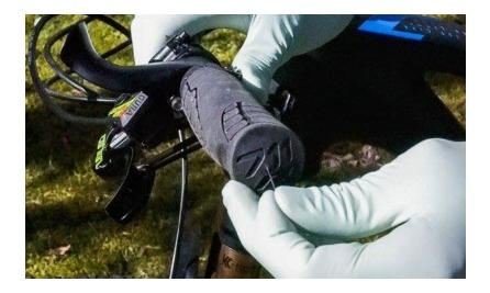
To do this, take a thin needle and prick the middle of the outside of the grip, thus allowing the air to escape. The rubber material then closes the hole by itself and prevents moisture from penetrating. Please make sure that the hole is not too large when you prick the grip, this is the only way to guarantee a good hold.
