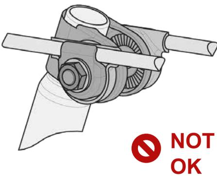
Clamping of the saddle frame with non-opposing clamping jaws or clamping surfaces is to be avoided in all cases. Otherwise, the saddle frame is subjected to a bending stress that can lead to premature failure or sudden breaking during use and thus to an accident.
