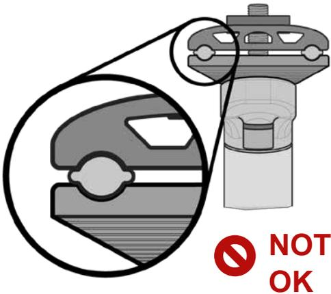
Observe the tightening torque of the saddle clamping stated in the operating instructions for your seat post. Never exceed the maximum tightening torque of 18 Nm. If there is a conflict between the torque specifications, please contact your dealer. This may lead to an impairment of product safety and damage with consequent breakage.
